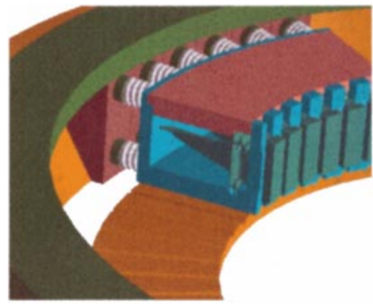
Fig. 14 Universal tool assembly allowing the spring or wedge approach
